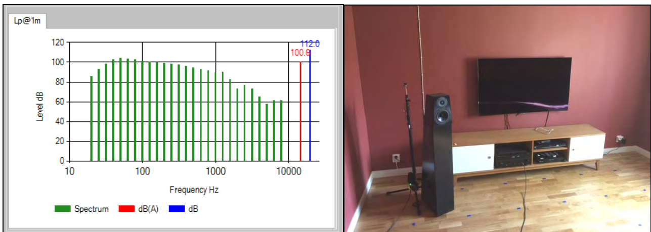
Figure 7: On the left, the 1/3 rd oct. band spectrum of the source derived from simulated narrow band values, while on the right shows the LF speaker used for the sound measurements.
