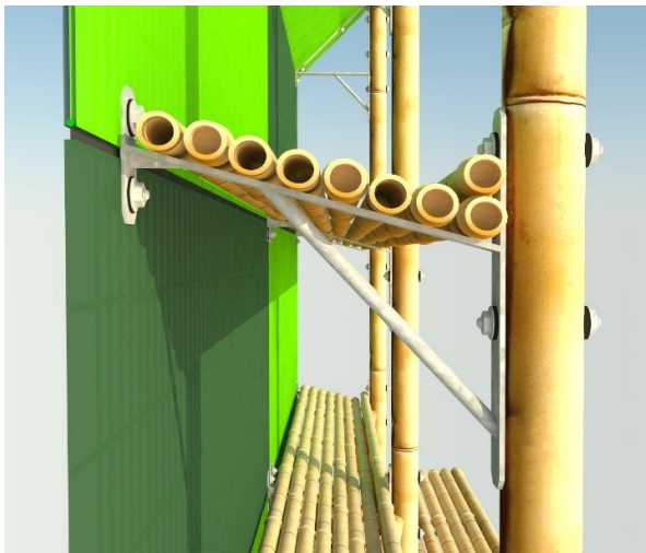
Fig.40. Bamboo Tray Typical Detail GMS Bracket Fixed to Treated Bamboo Frame Supporting PVA Screen.
